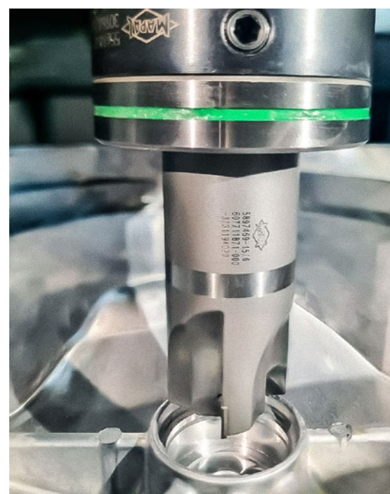
Finish machining tool with diameter 32 mm and PCD cutting edges for finishing the fitting bore with a P7 tolerance.
