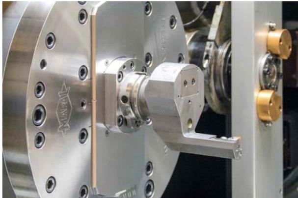
Two tailor-made single slide facing heads with automatic tool change, in conjunction with corresponding mounting tools, allow complex machining contours to be realised.
