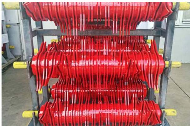
About a dozen different rollers and axles are required to build a round baler. This includes the rotor that is shown with welded-on teeth, which ensures optimum transport of the straw in the baler.
