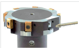
Fig. 4: Cleaning the insert pocket
