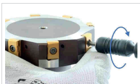
Fig. 7: Tightening the clamping screw
