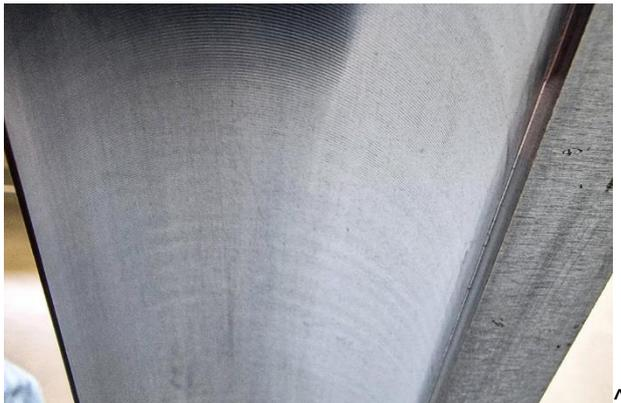
The further the robot arm extends, the greater the risk of vibration and chatter marks. Test series offer conclusions on cutting speed, feed and cutting depth for which a good surface is reliably produced with the milling cutter from MAPAL.
