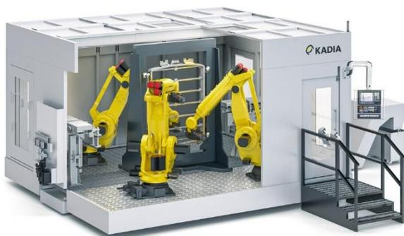
The custom machine layout requires the use of three robots. Two deburr the front, while the third machines the back. This achieves the optimum cycle rate in industrial production. ©KADIA Produktion GmbH + Co.
