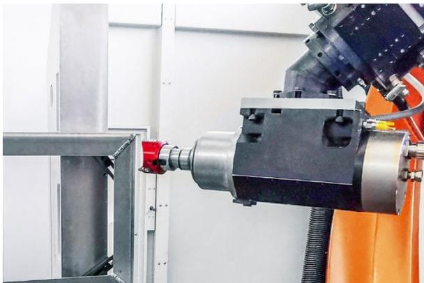
A dummy clamped in the test cell corresponds to half of an original part in its dimensions and material. In the tests, KADIA doesn't just determine the optimum cutting data, but also the most suitable position of the robot in relation to the workpiece. ©KADIA Produktion GmbH + Co.
