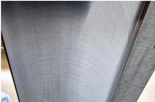
The further the robot arm extends, the greater the risk of vibration and chatter marks. Test series offer conclusions on cutting speed, feed and cutting depth for which a good surface is reliably produced with the milling cutter from MAPAL.
