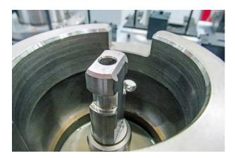
The actuation of the slides of the actuating tool are operated using a drawbar with a high-precision bayonet coupling.
