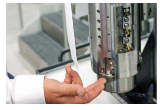
The run-out variation of the tool must not exceed 3  $\mu m$  for a length of 380 mm.
