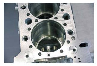
Maximum precision is required when machining the connections for the cylinder liners in lorry engine blocks.
