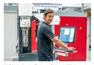
MAPAL Application Engineer, Christoph Wilhelm, on the measuring and setting fixture with suspended tool arrangement specially developed for this application.
