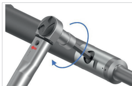
Fig. 16: Tightening clamping stud to tightening torque
