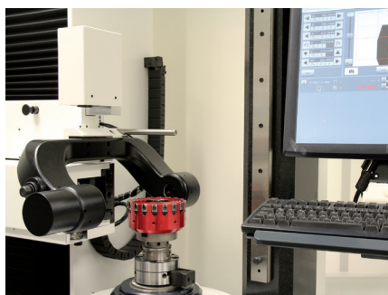
5. Use the setting fixture to optically set a milling cartridge -0.01\text{ mm} before the setting dimension (EM). To do this, measure the cutting edge with the optical measuring device and turn the threaded spindle clockwise with a hex-wrench until \text{EM} = -0.01\text{ mm} is reached. For purely optical setting, repeat this process for the remaining milling cartridges (then continue with step 7).
