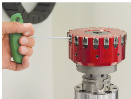
2. Loosen the clamping screw of the milling cartridge and remove it upwards from the dovetail guide.
