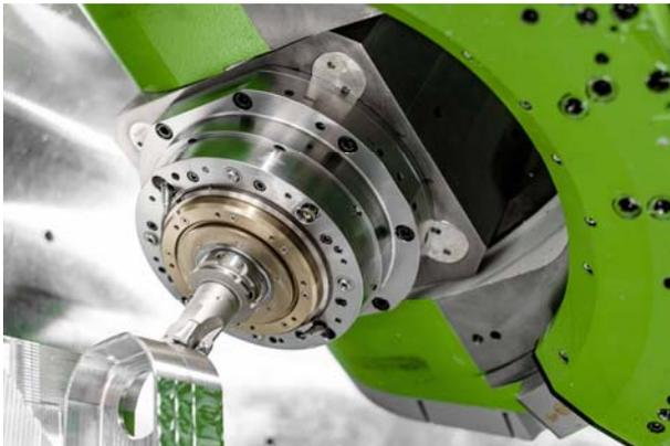
The horizontal machining centre, the 3-axis milling head and the ISO shoulder milling cutter SPM-Rough achieve best results when used together.
