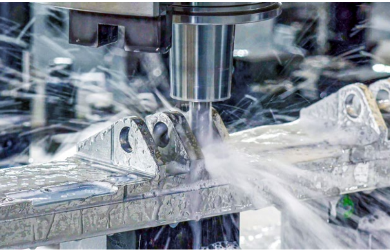
An OptiMill-HPC-Titan is used to machine the gaps between the lugs.
