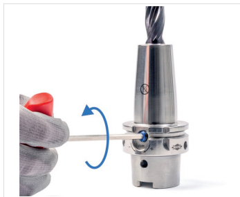
Fig. 14: Loosening clamping screw
