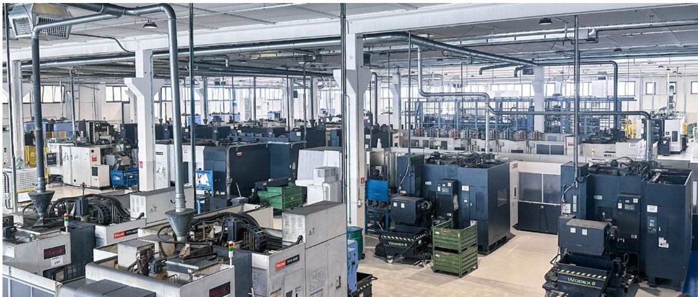
A total of 57 horizontal machining centres from MAZAK, MCM, MAKINO and DOOSAN are available for flexible manufacturing – as stand-alone machines, operated manually or by robot, and within FMS setups. ©Casappa S.p.A.
