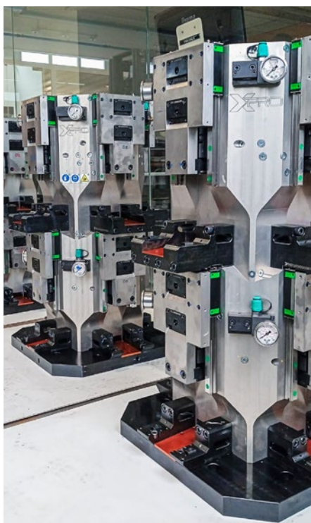
Clamping fixtures from the MAPAL Group add another key component to the turnkey offering within the process chain.
