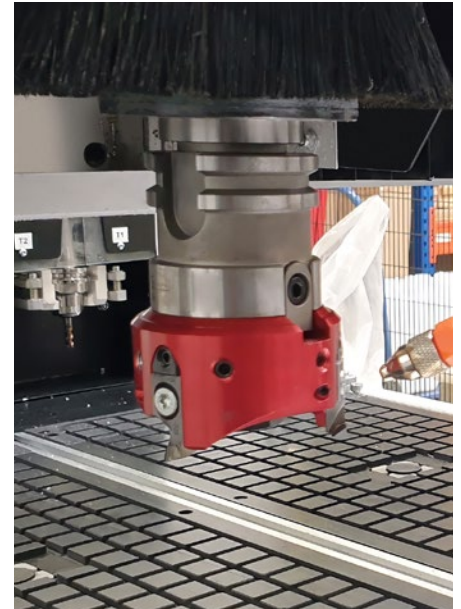
MAPAL's lightweight HSC NeoMill-Diamond-FlyCutter milling cutter is perfectly suited for machining the surfaces of plastic parts clamped by M-O-T on a vacuum table using a BT30 connection.
