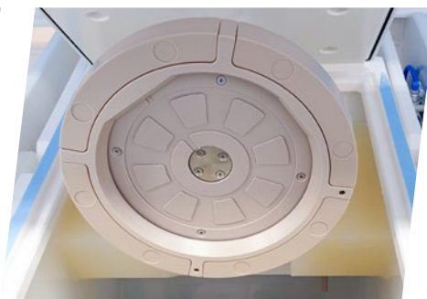
The process cells hold round silicon wafers supplied by users. These are then treated with chemicals as part of processes that can frequently last for hours.
