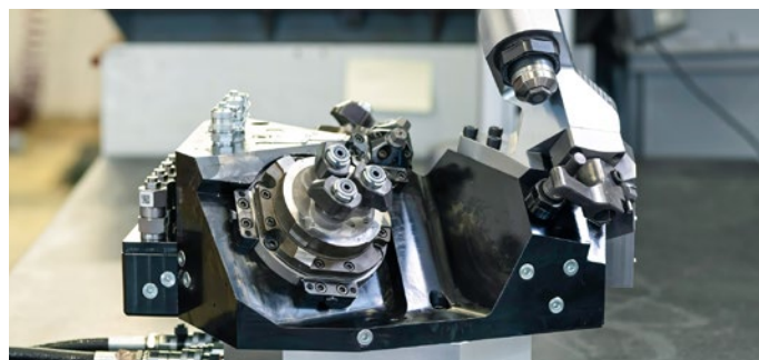
Hydraulic clamping fixtures are often used when high production quantities, short cycle times or automated processes are needed.
