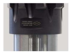
The gap between the replaceable head and replaceable head holder is closed and a joint with a force and form fit is formed. The replaceable head CPReam is now ready to use.
