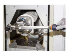
**4.**Place the torque wrench on the replaceable milling head so it is as horizontal as possible; do not tilt the faces on the spanner.
