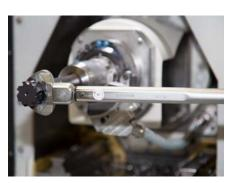
5.Tighten the replaceable head to the stated tightening torque with the aid of the torque wrench and the appropriate open-ended spanner attachment (see table "Tightening torques for the replaceable heads").
