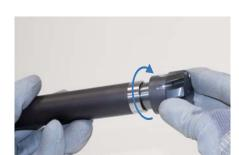
3.Screw the replaceable head clockwise into the replaceable head holder so it is hand-tight. Then clamp the replaceable head holder with the tool in the machine holder
