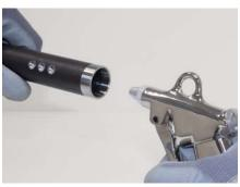
Clean the taper, thread and face surface on the replaceable head holder using compressed air and a cloth.
