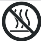
Fig. 1: Prohibition symbol on the hydraulic chuck
