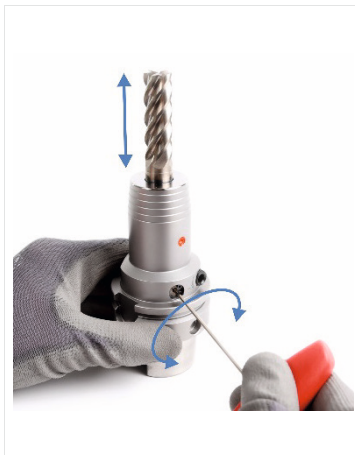
Fig. 11: Adjusting tool length (radial)
