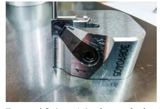
The cassette's flat bottom is the reference surface for quick and easy setting of the insert position. The setting dimension can also be found there. ©Klaus Vollrath
