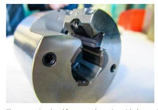
The conventional tool for external reaming with three guide pads and the indexable insert with one cutting edge. ©Klaus Vollrath
