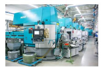
Multi-spindle automated lathes stand side by side in the machine hall. ©Klaus Vollrath
