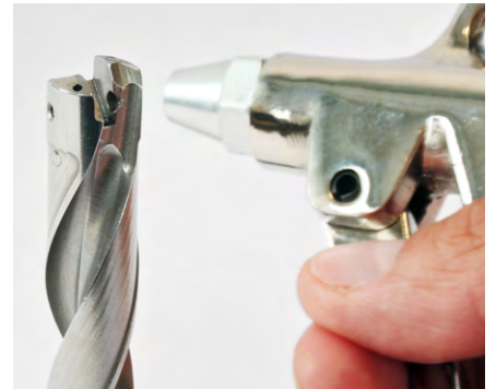
3. Clean the insert seat using compressed air.
