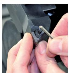
Step 1: Undo clamping
