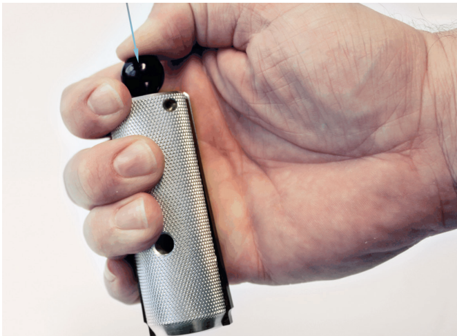
Opening the KS assembly tool
