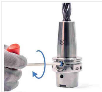
Fig. 13: Clamp the tool
