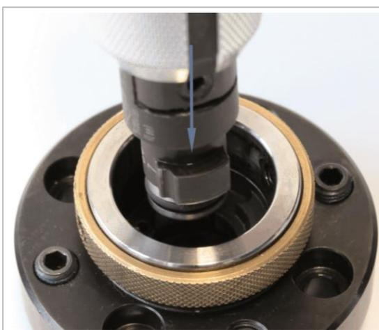
Fig. 6: Inserting the KS clamping cartridge
