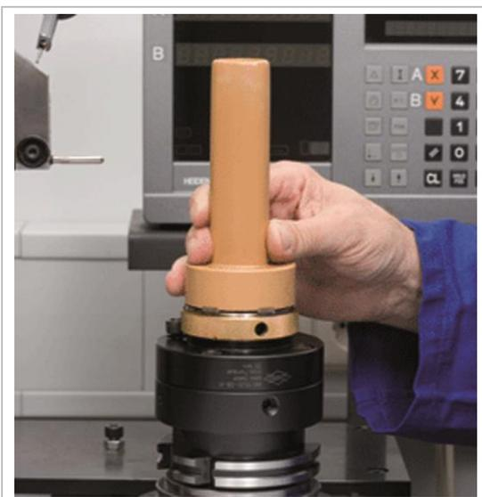
Fig. 8: Cleaning the HSK interface
