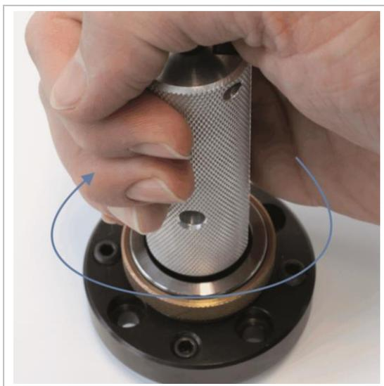
Fig. 7: Arresting the KS clamping cartridge
