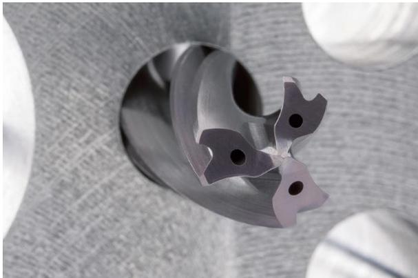
Drilling and reaming in one go: with a self-centring chisel edge and six guiding chamfers, the Tritan-Drill-Reamer with three cutting edges offers maximum process reliability with a variety of application parameters. ©MAPAL
