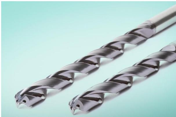
With 8xD and 12xD in stainless steel: forced orbital movements reduce the pressure on the three guiding chamfers of the MEGA-Speed-Drill-Inox. The flute core tapers towards the back and ensures reliable chip removal. ©MAPAL
