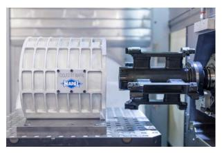
Using a fine boring tool as a welded design, the main bore of the central housing is machined to an accuracy of a few  $\mu$ m.
