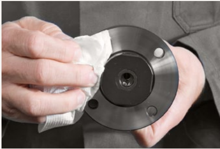
1. Clean taper and face surfaces on the flange adapter and adapter.
