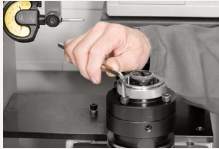
2. Insert flange adapter. Tighten fastening screws to 50 % of the tightening torque stated (see table).
