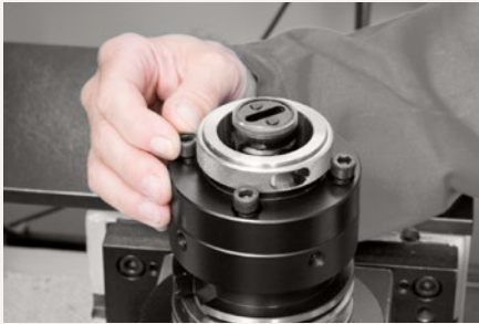
2. Insert flange adapter. Tighten fastening screws to 50 % of the tightening torque stated (see table).
