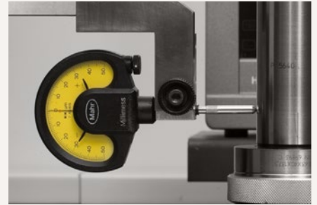
5. Place dial gauge in contact at the position for the radial run-out check. On MAPAL tools it is also possible to use the HSK collar for alignment. Take highest measuring point and set dial gauge to "zero".
