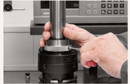
4. Insert test arbor or tool and fasten using clamping screw.
