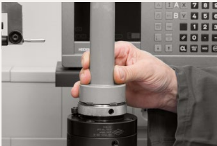
3. Clean taper and face surface on test arbor or tool.
