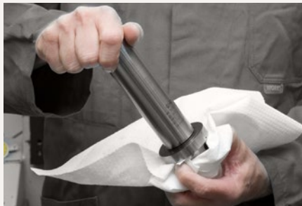
2. Insert flange adapter. Tighten fastening screws to 50 % of the tightening torque stated (see table).
