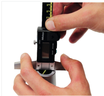
Fig. 6: Set shrink chuck to tool length
