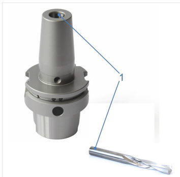
Fig. 5: Clean the shrink chuck and tool
