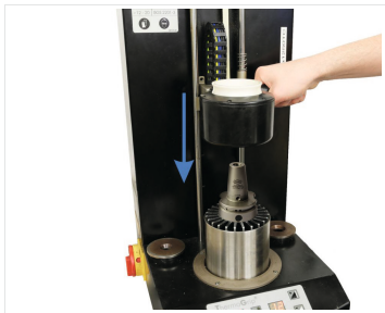
Fig. 7: Heat the shrink chuck with shrink unit
