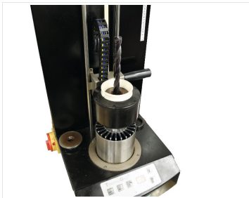
Fig. 10: Heat the shrink chuck with tool
