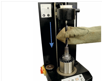
Fig. 8: Insert tool into the location bore
