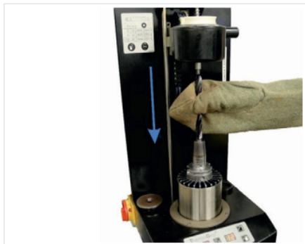
Fig. 8: Insert tool into the location bore
