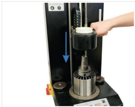
Fig. 7: Heat the shrink chuck with shrink unit
