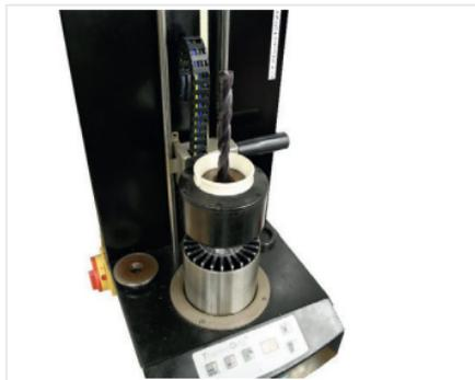
Fig. 10: Heat the shrink chuck with tool
