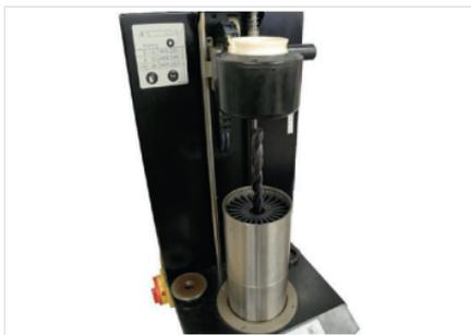
Fig. 9: Cool the shrink chuck with tool
