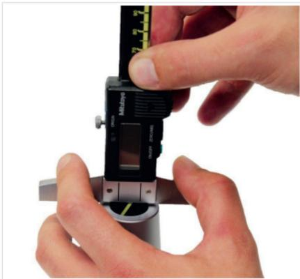
Fig. 6: Set shrink chuck to tool length
