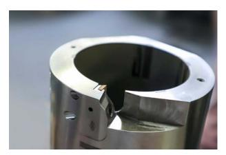
With the external reamer, a cylindrical form deviation of less than 5  $\mu m$  is reliably achieved.
