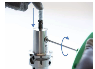
Fig. 4: Press on the tool and tighten the clamping screw
