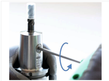
Fig. 6: Loosening clamping screw
