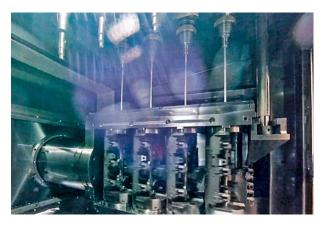
Quadruple machining of fuel-supply distributor parts with deep drills. The clamping fixtures that rotate in opposite directions to minimise the deviation of the drill are what makes the solution exceptional. Photo provided by ELHA.
