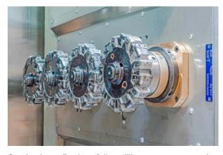
Quadruple application of disc milling cutters on control arms. The solid cutting surfaces provide an indication of the high drive power required. Photo provided by ELHA.
