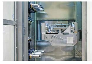
A peek inside the interior of a manufacturing module shows that it features two spindle row revolvers, left.
