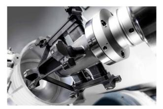
In order to produce the main bore of the stator housing with  $\mu m$  accuracy, it is machined with a fine boring tool from MAPAL. Bild: HELLER
