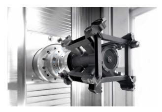
The tool concept is impressive, among other things, thanks to its low weight and the finely adjustable PCD cutting edges
