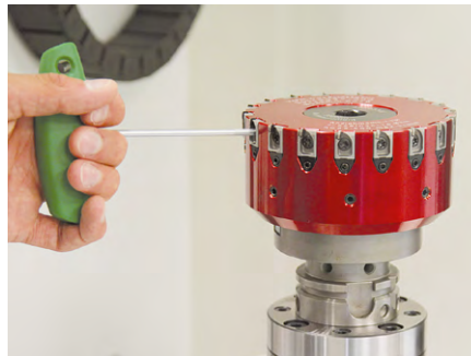
2. Loosen the clamping screw of the milling cartridge and remove it upwards from the dovetail guide.
