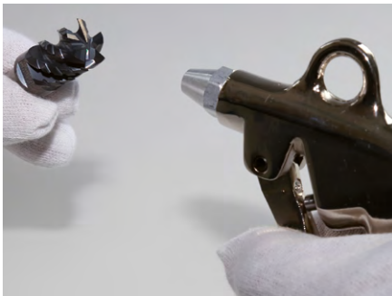
1. Clean the taper, thread and face surface on the replaceable milling head using compressed air and a cloth.
