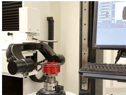
5. Use the setting fixture to optically set a milling cartridge -0.01\text{ mm} before the setting dimension (EM). To do this, measure the cutting edge with the optical measuring device and turn the threaded spindle clockwise with a hex-wrench until \text{EM} = -0.01\text{ mm} is reached. For purely optical setting, repeat this process for the remaining milling cartridges (then continue with step 7).
