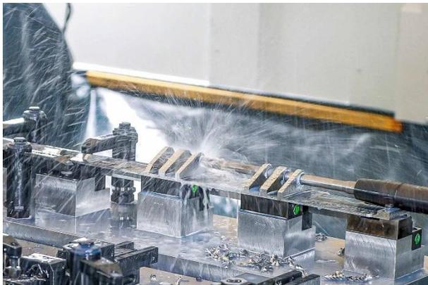
A special design of the MEGA-Speed-Drill-Titan carries out the pre-machining of the main bore of the second lug pack. The tool is led through the first lug pack.
