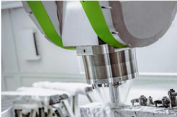
The outer contour is preroughed on the six-axis FZ42 with a VH60 milling head with a NeoMill-Titan. © F. Zimmermann GmbH
