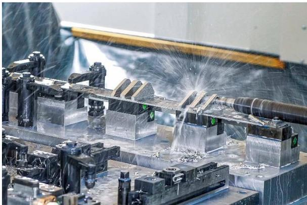
The main bore of the first lug pack is piloted by the MEGA-Speed-Drill-Titan.
