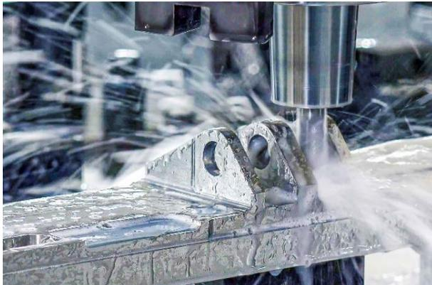
An OptiMill-Titan-HPC is used to machine the gaps between the lugs. ©MAPAL
