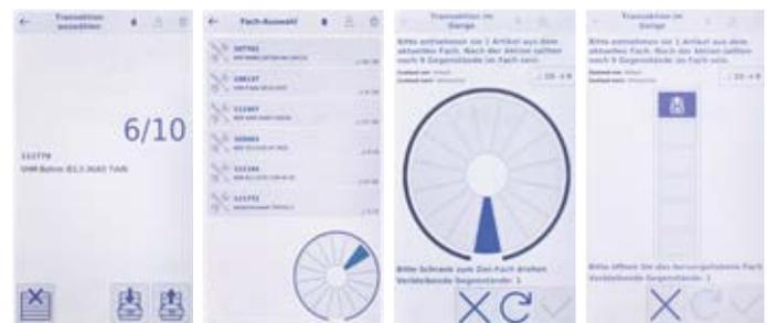
Easy to use: After the desired transaction has been selected, the drum position is shown. After turning the drum by hand, the compartment is marked with a blue light bar and can be opened. Finally, the transaction must be acknowledged.
