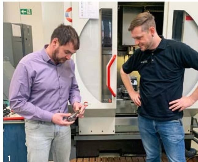
**1** After initial tests for roughing a slide, Managing Director Marco Schülken and Manufacturing Manager Marcus Vogt inspect the tested MAPAL NeoMill-4-HighFeed-90 high-feed milling cutter.
