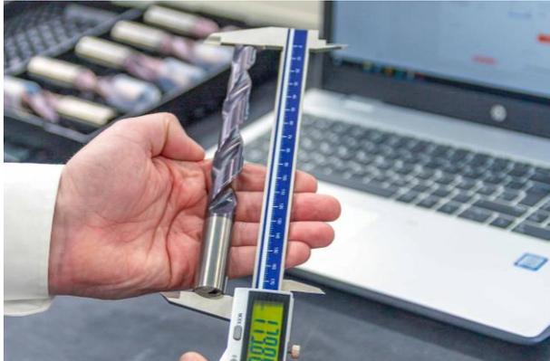
At just the touch of a button, measurement results are transferred from the Bluetooth caliper to c-Com.
