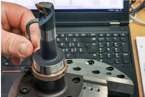
The turning tool is mounted on the slide. © MAPAL
