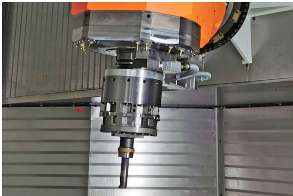
The mechatronic tool system TOOLTRONIC, installed in the milling-turning centre RX18 of the Reiden Technik AG. © MAPAL
