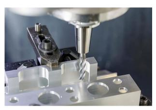
The solid carbide milling cutter OptiMill-SPM-Finish finishes large pockets in a single pass.
