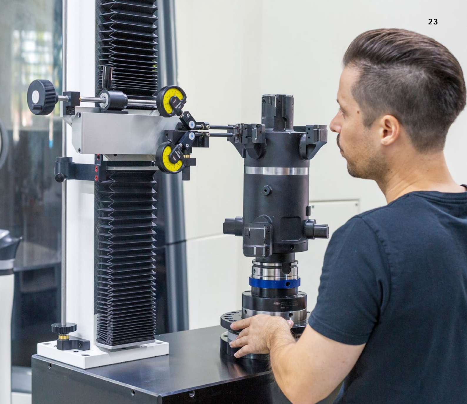
The UNISET-V basic plus is ideal for ultra-precise setting of guide pad tools with a diameter of 100 to 400 mm and a maximum measuring length of 750 mm.
