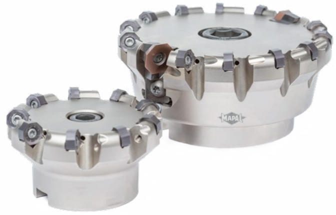
Unique and with complete process reliability – the NeoMill-16-Finish (right) with pre-machining insert ONMU05 with 16 cutting edges and indexable insert with eight cutting edges for finishing steel and cast-iron materials. The NeoMill-16-Face (left) offers efficient pre-machining for face milling.
