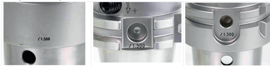
Fig. 6: Marking for checking of the clamping force: Three possible positions on the clamping chuck
