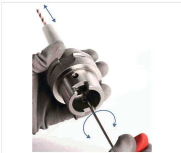
Fig. 10: Adjusting the tool length
