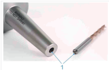
Fig. 8: Cleaning hydraulic chuck and tool
