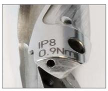
**5.** Tighten the special clamping screw to the stipulated tightening torque.
