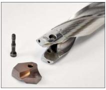
**2.** Remove the indexable insert from the insert seat.
