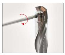
4. Fit the new indexable insert in the insert seat. Tighten hand-tight the special clamping screw with the aid of the TORX® PLUS wrench supplied by turning clockwise.
