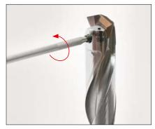
Undo the special clamping screw with the aid of the TORX® PLUS wrench supplied by turning counter clockwise.
