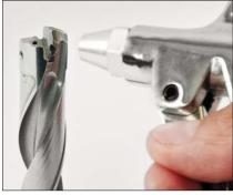
**3.** Clean the insert seat using compressed air.
