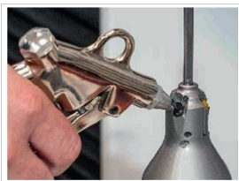
Fig. 6: Cleaning the insert seat
