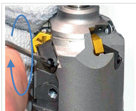
Fig. 18: Tightening clamping screw
