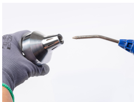
2. Clean the taper and contact surface on the replaceable head holder using compressed air and a cloth.
