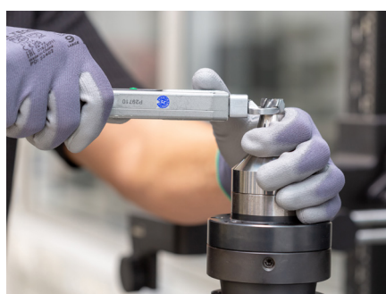
5. Tighten the replaceable milling head using the torque wrench and the corresponding combination wrench at the specified tightening torque (see table "Tightening torque of replaceable milling head").
