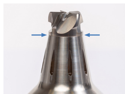
3. Hand tighten the replaceable milling head clockwise into the replaceable head holder. Then clamp the replaceable head holder with the tool in the setting fixture or an assembly system.
