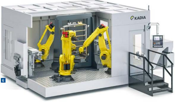
the more unstable the machining. That's why KADIA doesn't just test various cutting data, but also various positions for the robot, in front of or beside the workpiece.
