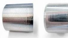
Comparison of the typical surface of a turning workpiece (left) with a sleeve finished using external reaming.
