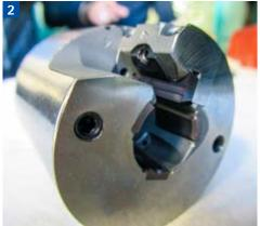
2 The conventional tool for external reaming with three guide pads and the indexable insert with one cutting edge.
