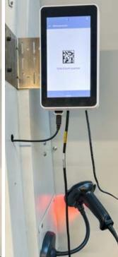
Two of the EMCO machines are equipped with c-Connect boxes for transferring data via scan to the machine.
