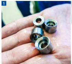
1 Some turning workpieces still oiled straight from the machine.
