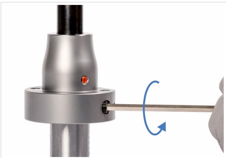
Fig. 17: Loosening clamping screw
