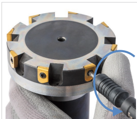
Fig. 2: Releasing the clamping screw
