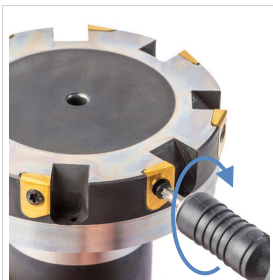
Fig. 6: Tightening the clamping screw
