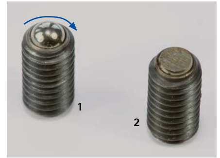
3. Check whether the flat side of the locking screw (2) is pointing in the direction of the milling cartridge. If a spherical shape can be seen (1), use your finger to turn this to the flat position.
