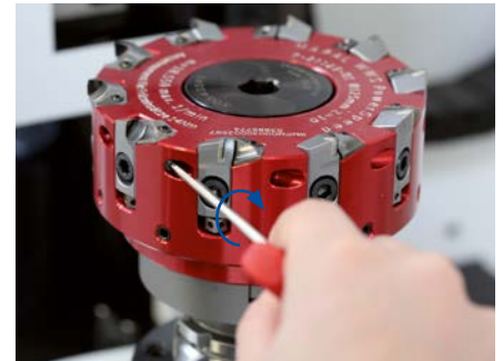
6. Screw in the locking screw clockwise to the stop using a hex-wrench and then screw back half a turn.
