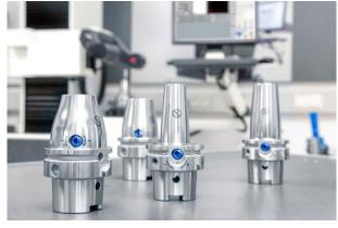
Simple and straightforward handling is a further advantage of hydraulic clamping technology. ©MAPAL
