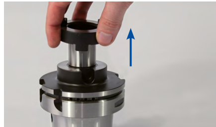
1. Remove the driving ring from the milling cutter arbor.
