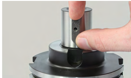
2. Insert the feather key on the milling cutter arbor.
