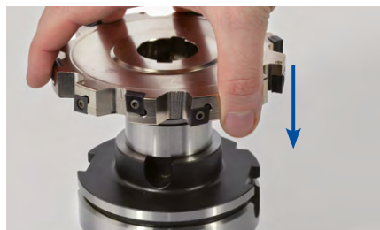
5. Place the tool flat on the milling cutter arbor.
