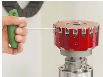
2. Undo the clamping screw for the milling cartridge and remove upward out of the dovetail guide.
