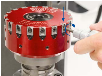
4. Note: Press the milling cartridge lightly while tightening such that the adjusting wedge is in contact.
