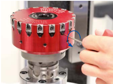
1. Turn the threaded spindle one turn counter-clockwise using a hex-wrench with a wrench size of 2.5.
