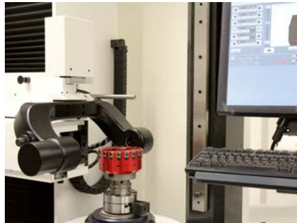
5. Using the optical setting fixture, set a milling cartridge -0.01 mm in front of the setting dimension EM: For this purpose reach the cutting edge using the optical measuring device and using a hex-wrench turn the threaded spindle clockwise until EM = -0.01 mm is reached. For purely optical setting, repeat this process for the remaining milling cartridges (then continue with step 7).
