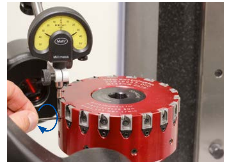
6. Position the dial gauge on the milling cartridge and set to zero. Using the dial gauge set the milling cartridges to -0.01 mm in front of EM: For this purpose turn the threaded spindle clockwise using a hex-wrench until the zero dimension is reached.
