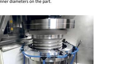
In simultaneous machining, the workpiece is moved into the annular gap between the outer tool and the inner tool from above. Plenty of cooling lubricant is used for machining. © NILES-SIMMONS-HEGENSCHEIDT GmbH
