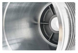
Machining the stator housing includes internal machining with various sections, machining the smaller centre bore and machining the outside with its cooling ribs.
