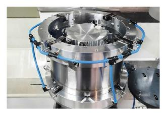
The semi-finishing tool for inner machining is clamped in the lower spindle. It is surrounded by the bell-shaped outer tool, which is securely mounted.
