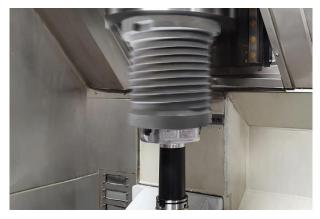
The first step is roughing the inside of the housing.
