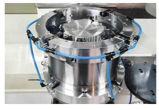
The semi-finishing tool for inner machining is clamped in the lower spindle. It is surrounded by the bell-shaped outer tool, which is securely mounted.
