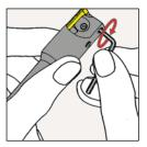
5. For coarse setting, turn the front and rear threaded pin one quarter of a turn clockwise.
