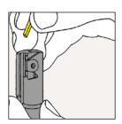
3. Remove the indexable insert. Clean the indexable insert and the indexable insert seat (do not use compressed air, pay attention to adjusting wedge). Rotate the indexable insert or fit a new indexable insert.
