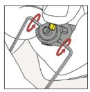
4. Note: Two wrenches must be used for tightening. Press the indexable insert and the cassette against the rear stop and the adjusting wedge. Tighten the TORX® screw or the threaded spindle clockwise from above and counterclockwise from underneath and tighten.
